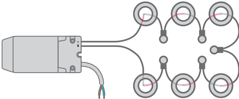
In a **parallel circuit**, all the components receive the same voltage across them but the current passing through may be different depending on the characteristics of each component.
