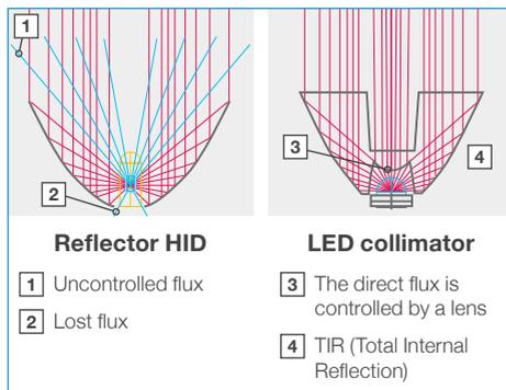
Note that collimator is high grade optical plastic and has lower losses than light reflecting off polished aluminium.
